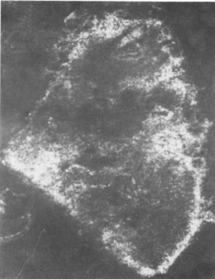
Fig. 15. Morphology of a single crystal which very often occurs in the carbon layer on adsorbent A2 (magnification 20 000 \times ).
