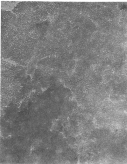
Fig. 3. Carbon layer deposited on adsorbent A2 (magnification 20 000 \times ).
